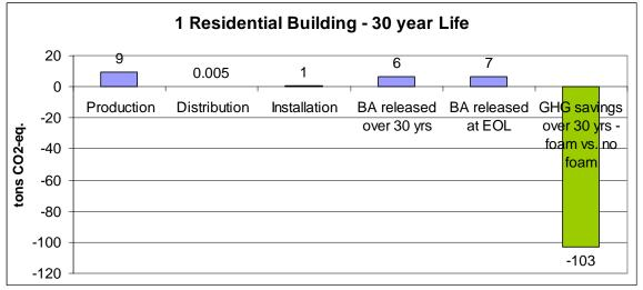
Figure 5 Residential Building: XPS Foam Life Cycle Impacts vs. Use Phase Savings
